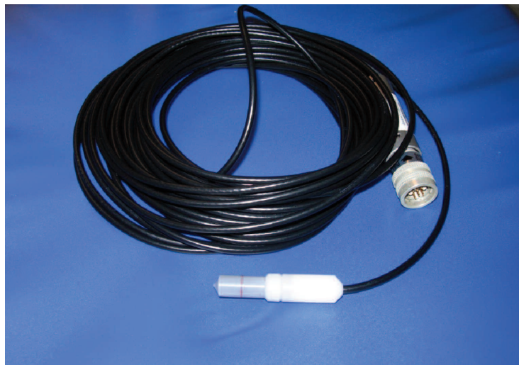
Figure 5. RadCal “Farmer-type” 0.6-cm 3 ionization chamber and cable. The red line along the circumference of the chamber locates the middle of the charge-collection volume.
