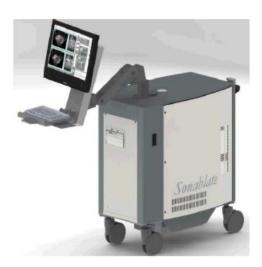
The Sonasource Console contains the system computer and electronics for HIFU planning and delivery. The monitor displays all system, patient, imaging, and HIFU delivery information via a graphical user interface. The keyboard and trackball are used for data and user-command entry. The trackball allows the operator to define the dimensions of the target zone and to measure the tissue distance from the rectal wall to the center of the target zone.
