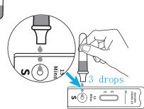
Invert the collection tube with sample, squeeze and add <u>3 drops</u> to the sample well of the test cassette.
