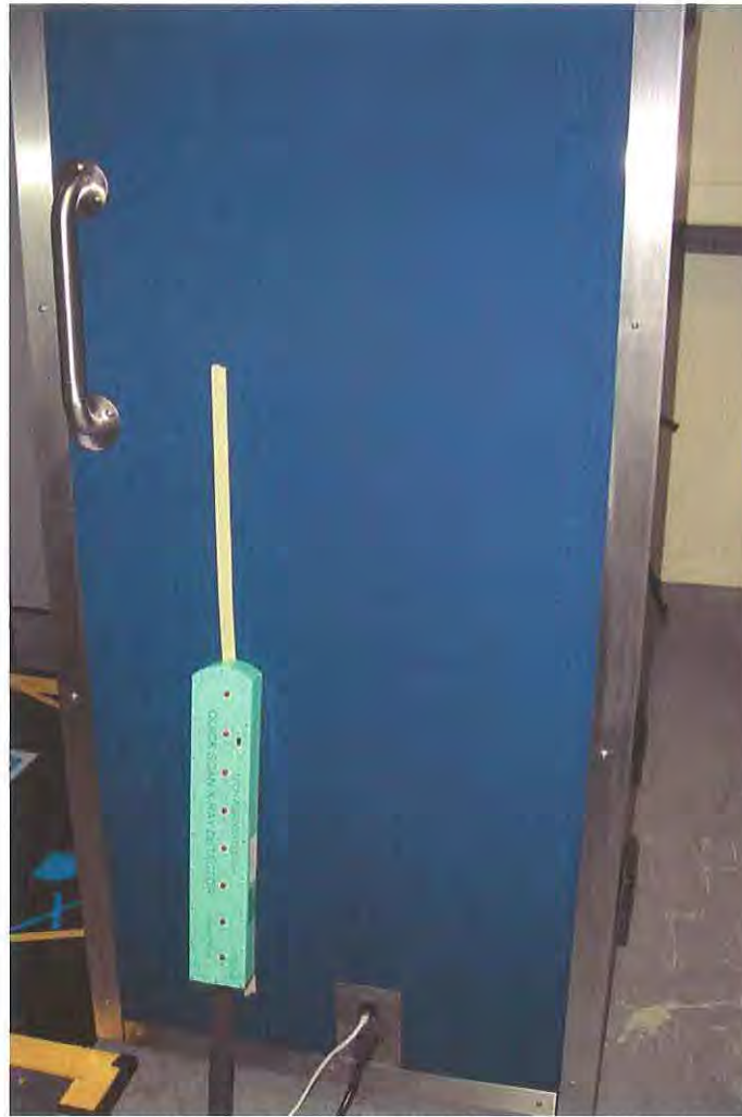
Figure 11. The P8-Neon detector and the tape marking the point of highest radiation leakage.
