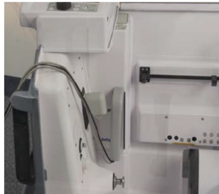
Figure 5: OCS™ Lung System Probes Pulled to the Side of the LPM
