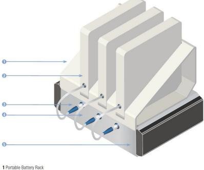
2 Portable Battery 3 Charger Socket 4 Charge Indicator 5 Charger
