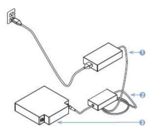
1 Plug-In Power Supply 2 Filter Box 3 the Device
