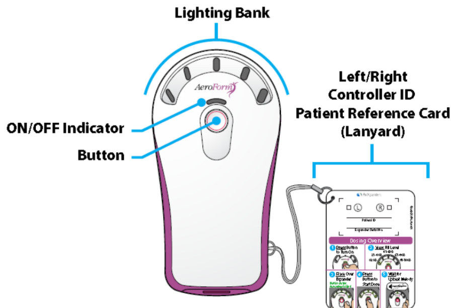
Figure 2: Schematic of Dosage Controller
