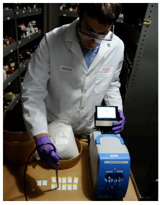
The results from the portable instruments are being verified by retesting samples with traditional laboratory analyses. In ongoing pilot programs, five portable ion mobility devices used for identifying dietary supplements containing undeclared drug ingredients have successfully been deployed across the United States.
