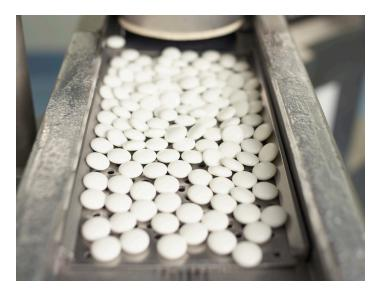
A very precise manufacturing "recipe" is established to get a consistent drug product. For example, a certain amount of ingredient must be added at the right time and/or temperature during the process. However, not all steps in the manufacturing process are equally critical to the quality of the final drug product. Therefore, it is important to most tightly control those ingredients and steps that have the greatest effect on drug behavior in the body.
