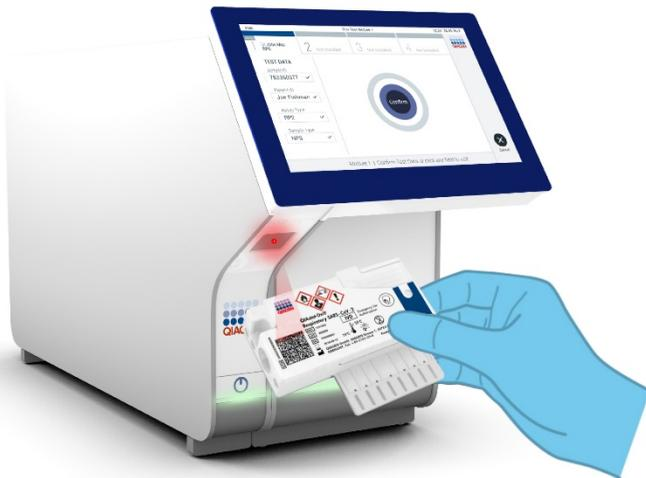
**Figure 12. Scanning QIAstat-Dx Respiratory SARS-CoV-2 Panel Cartridge bar code.**
