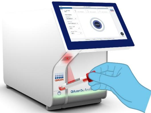
**Figure 11. Scanning sample ID bar code.**
