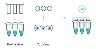
6. The void filling caps may feel slightly loose, this is normal. The thermocycler lid will secure the caps into place when closed, sealing each PCR reaction. **DO NOT** attempt to push the cap down.
