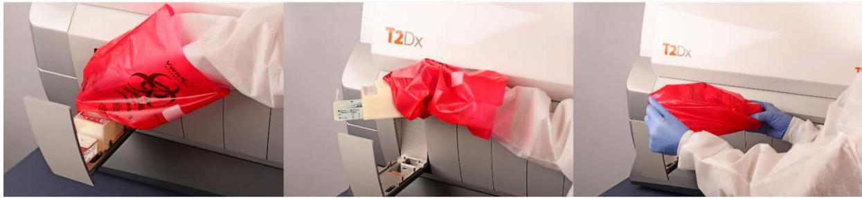
Figure 6. Proper Technique for Unloading the T2SARS-CoV-2 Panel.
