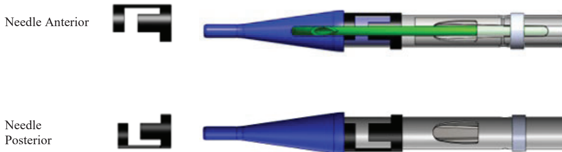
Figure 8: Crown Marker Band System Needle Direction (Directions are noted from the perspective of the device in a supine patient)
