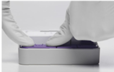
D. Push Button 3 all the way down to pierce the reagent seals. Use two thumbs, push firmly.
