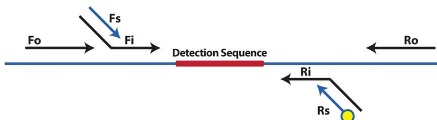
**Figure 1. Reaction Process.** Low concentration nested gene-specific primers are (Fo – forward out; Fi – forward in; Ri – reverse in; and Ro – reverse out) designed to enrich the targets during the initial PCR cycles. Later in the procedure, a pair of universal SuperPrimers (Fs and Rs) is used to amplify all targets. The Rs primer is labeled with biotin for subsequent detection.
