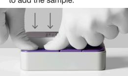
Push Button 3 all the way down. Use two thumbs, push firmly. Note: All buttons should be all the way down.
