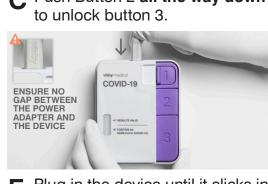
Plug in the device until it clicks into place. A stable white light indicates the test is running.
