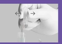
F Keep the tip fully under the fluid. Release the upper bulb.
