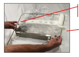
Inserting rails into outer sleeve of the isolette.
