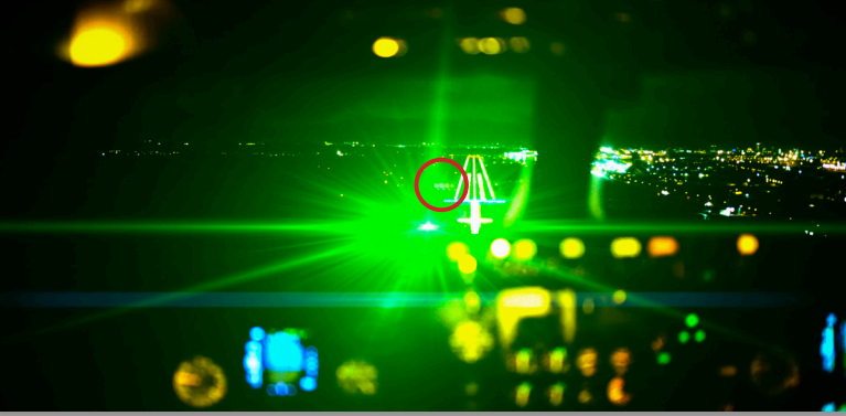
Figure 1: Laser illumination in a flight simulator as viewed from the pilots' perspective approximately a mile away at least above ground level. The circle to the right of the flash contains runway lights
