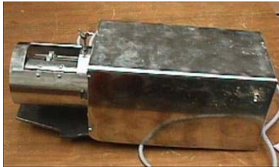
Figure 23 – Mechanical stainless steel oyster grinder
