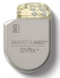
Figure 2: Implantable Pulse Generator
