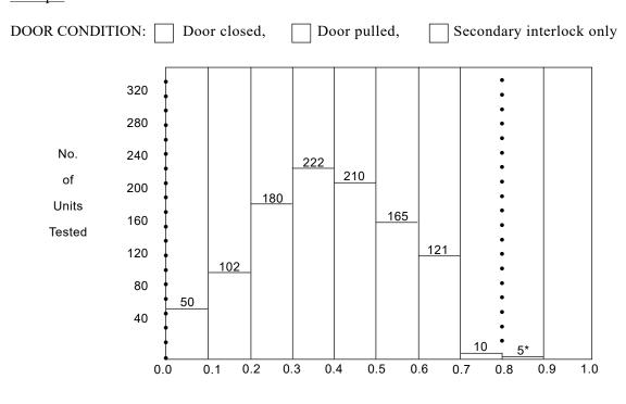
Microwave Leakage (mW/cm<sup>2</sup>) for model family AB
