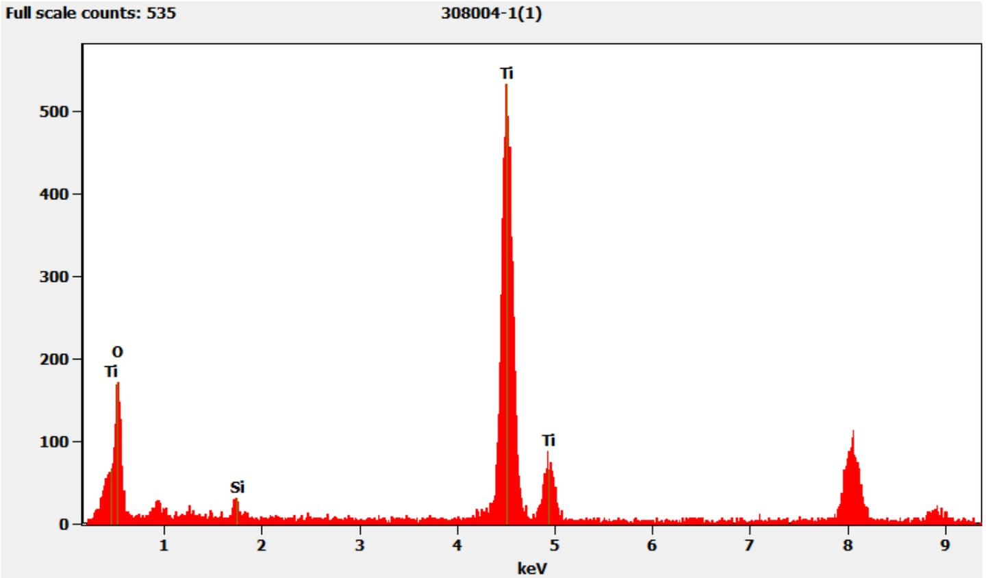
Particle coated with Titanium from 308004-1
