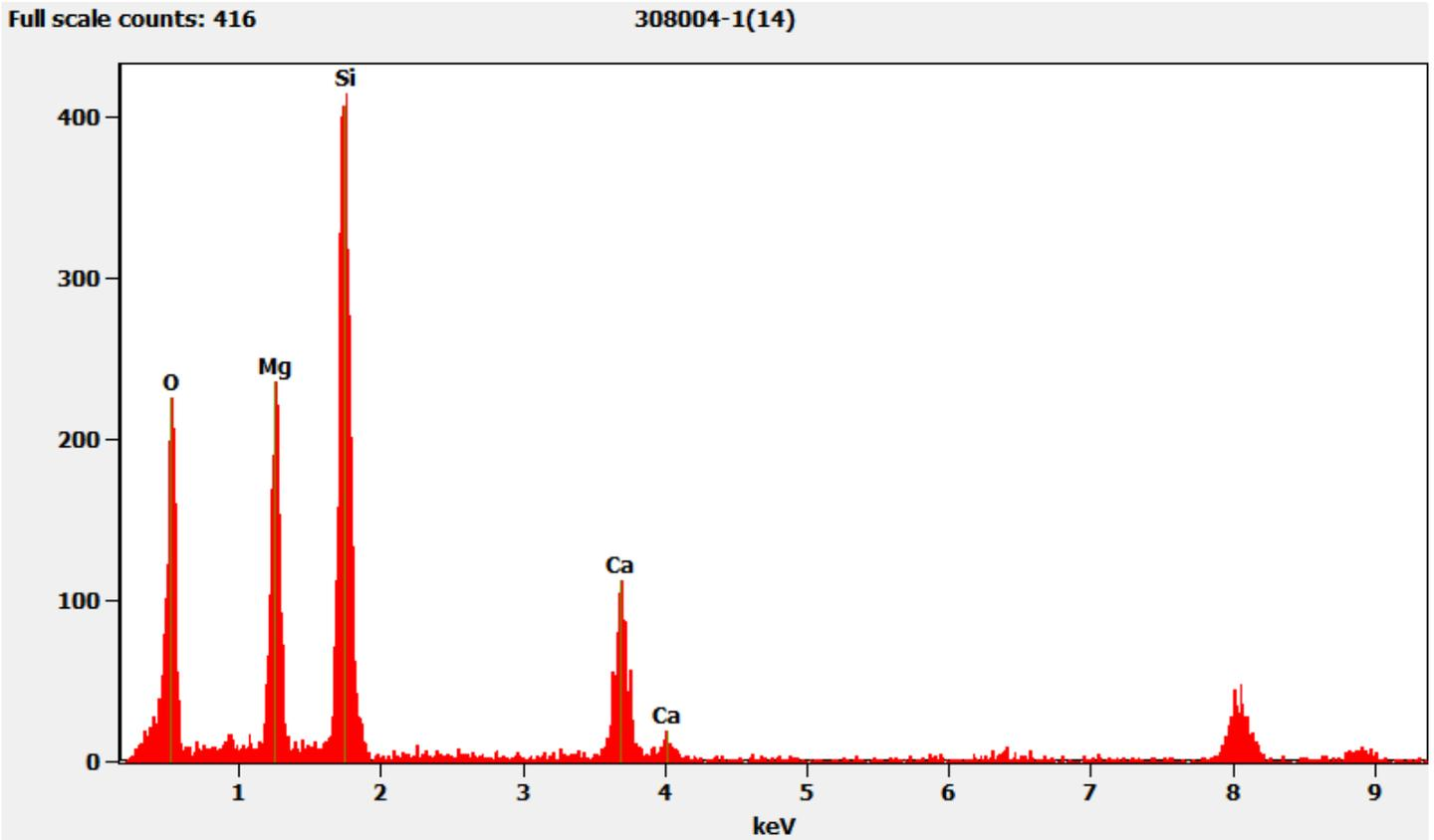
Tremolite Particle from 308004-1A
