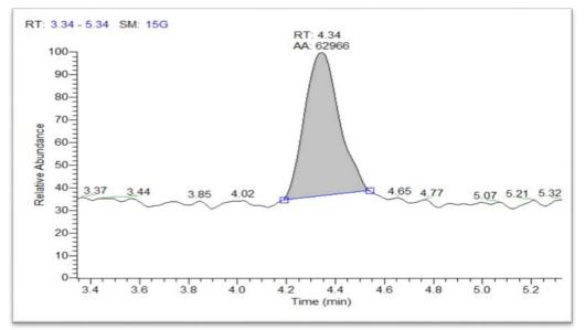
Extracted ion chromatogram of m/z 75.0553 from PRM scan of m/z 75.0553 at a mass accuracy of 15 ppm
