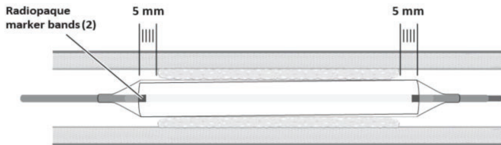
Figure 5. Centering of the stenosis within the SurVeil DCB radiopaque marker bands
