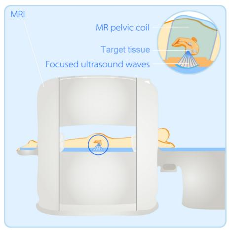
Fig. 1: The basic principles of MR-HIFU
