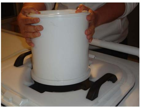
**Fig. 100:** Place one edge of the QA phantom on the phantom plate. Gently lower the QA phantom onto the phantom plate.
