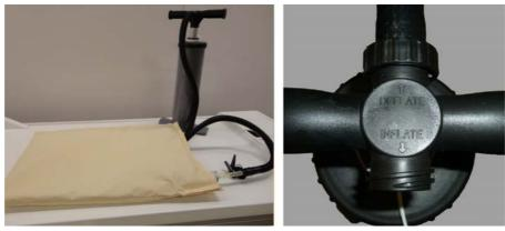
**Fig. 112:** Air pump. Right: Air hose connected to the Deflate side of the handle.
