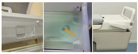
**Fig. 8:** Left: Tabletop release handle. Middle: The emergency tabletop release button located in the accessory box. Right: The emergency tabletop release handle located on the side of the accessory box.
