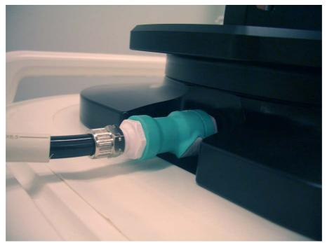
4. Connect the other end of the filling hose to the female hose connector in the Sonalleve tabletop.
