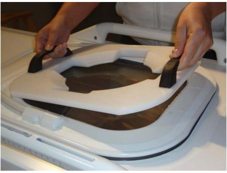
Fig. 99: Placing the QA Phantom Plate over the ultrasound window.
