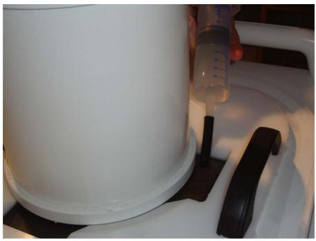
Fig. 101: Fill any remaining air pockets under the phantom with degassed water.
