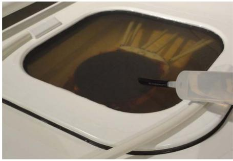
**Fig. 97:** Preparing the Sonalleve Tabletop with degassed water for phantom.
