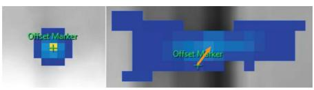
**Fig. 83:** If the offset marker does not appear at the center of the heating, drag the offset marker to the center of the heating manually.
