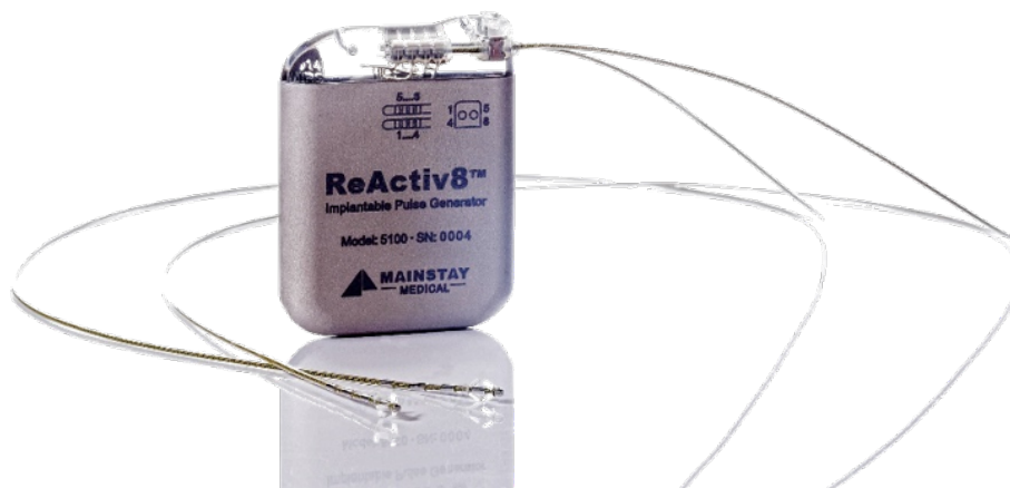
Figure 1: ReActiv8 Neurostimulation System Implantable Pulse Generator (IPG) and Percutaneous Leads
