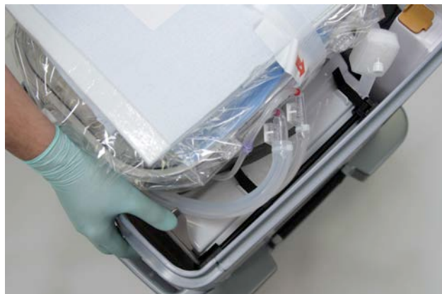
Figure 32: Press LvPM Back to Engage the Holding Clamps on Back Wall of the Liver Console
