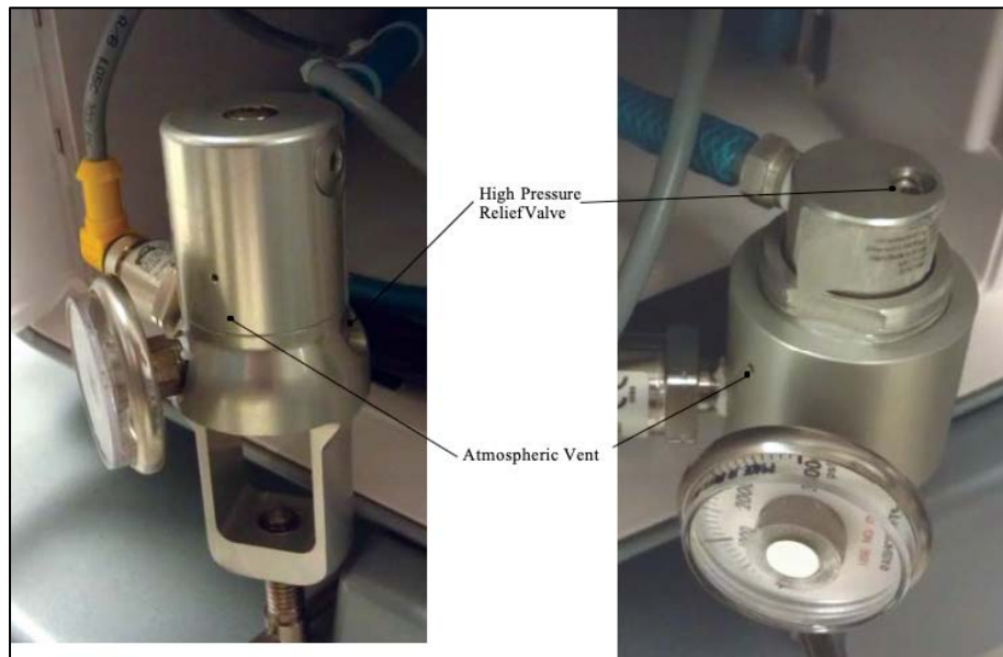
Figure 1: Left: CPI Regulator (note smooth body); Right: PI Regulator (note threaded body)
