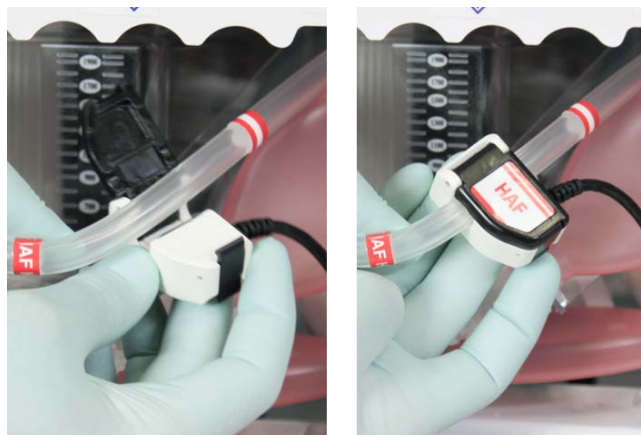
Figure 37: Insert Tubing Into Probe and Close Cover
