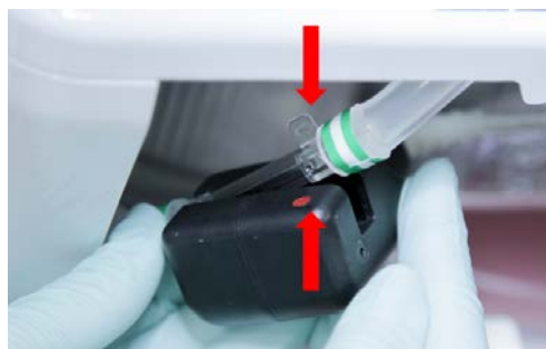
Figure 40: Align SvO 2 /HCT Probe with Cuvette on Tubing
