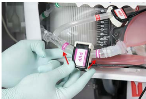
Figure 35: Probe and Tubing Labeled with Matching Colors (Purple in this Example)
