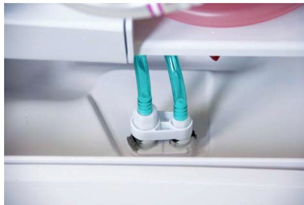
Figure 34: Gas Lines Connected
