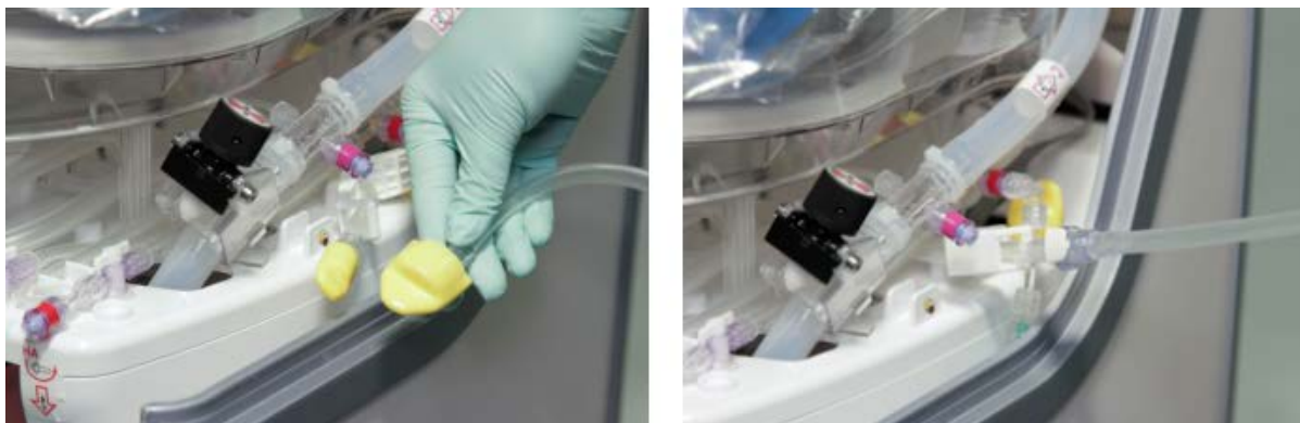
Figure 49: Connect the Prime Line to the LvPM
