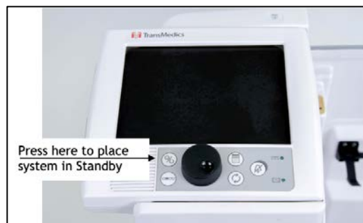
Figure 25: Press Power Button on Wireless Monitor
