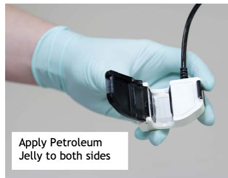
Figure 36: Open Probe Cover and Apply Petroleum Jelly
