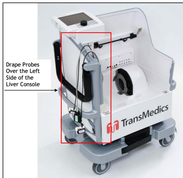
Figure 28: Prepare Liver Console for LvPM Installation
