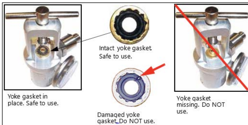
Figure 70: Gas Cylinder-Regulator Yoke Gasket
