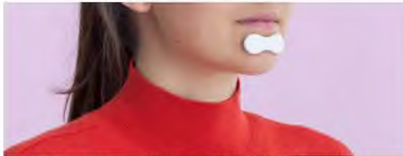
Figure 1 Sunrise Sensor Placed on Mandible
