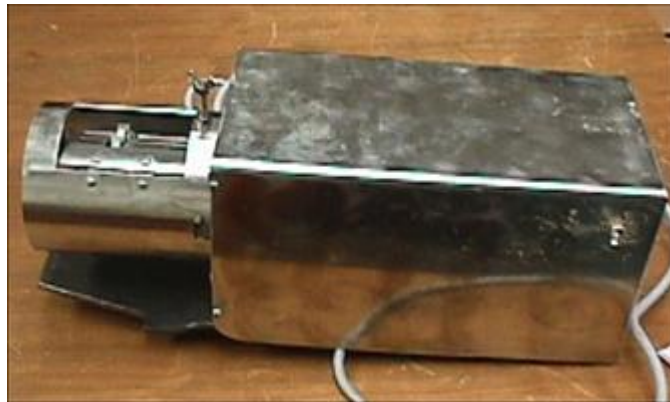
Figure 23 – Mechanical stainless steel oyster grinder
