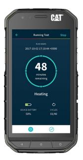
Biomeme Go (REF# <u>1000013</u> or REF# <u>1000012</u>) is an intuitive smartphone app that pairs wirelessly with the Franklin<sup>™</sup> real-time PCR thermocycler. It is compatible with Android 6.0.0+. The easy-to-use interface allows you to run, monitor, and analyze your tests online or offline and quickly interpret your results. Follow the simple steps outlined below to begin your test.
