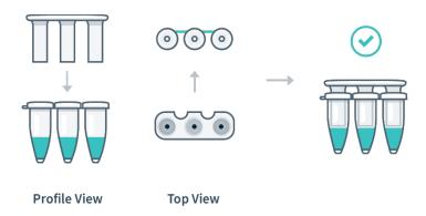
7. The void filling caps may feel slightly loose, this is normal. The thermocycler lid will secure the caps into place when closed, sealing each PCR reaction. **DO NOT** attempt to push the cap down.
