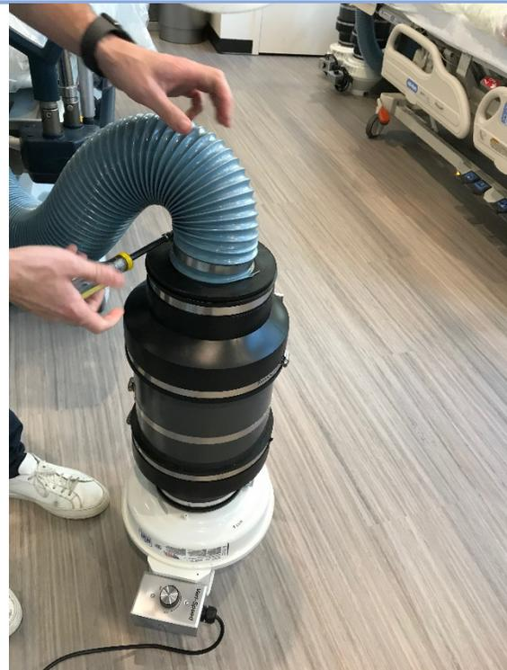
4. Remove screw from the hose clamp connecting the black top filter case to the main grey filter case using a screwdriver.
