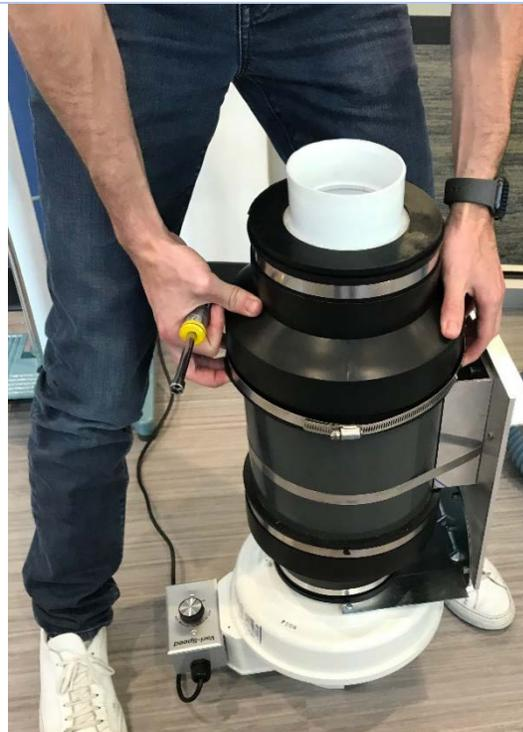
6. As the top case is lifted, the filter should be visible. Once the filter is free from the filter case, open a biohazard bag, hold the filter inside the bag, and use the bag to grasp the filter.
