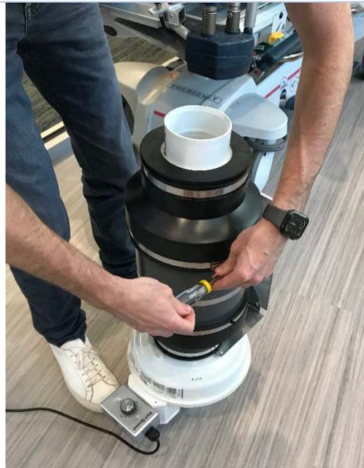
5. Slide the loosened hose clamp down. Remove top black filter case.
