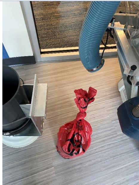
8. Loosen hose clamp holding white filter adapter and black case together, remove white adapter and dispose of it in biohazard bag.
