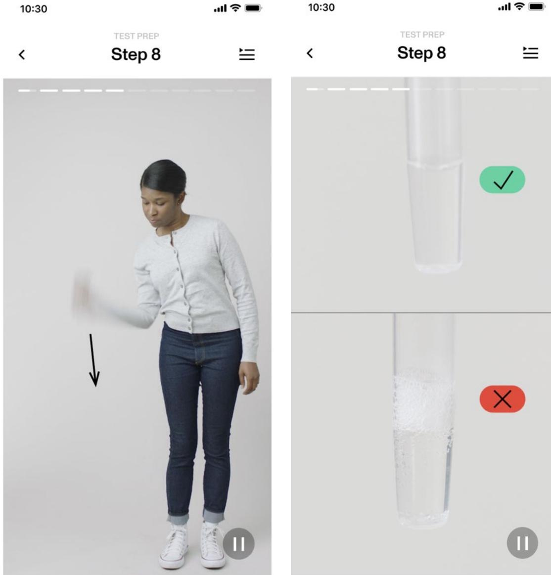
**REMINDER:** Liquid clinging to tube walls or cap may result in an invalid test.
