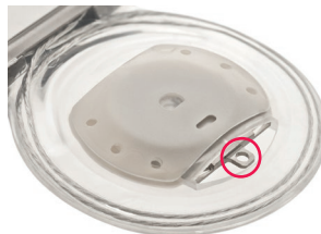
Figure 25: Metal tab on magnet cassette
