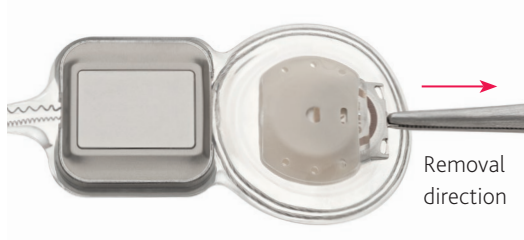
Figure 26: CI622 implant magnet cassette removal using metal tab
