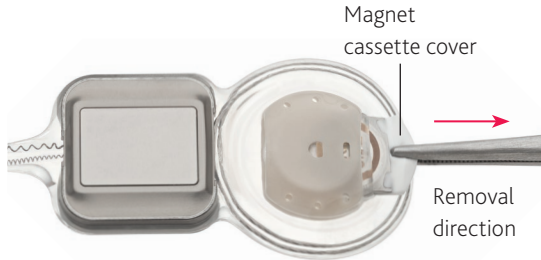
Figure 25: CI624 implant with magnet cassette partially removed
