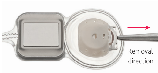
Figure 20: CI612 implant magnet cassette removal using metal tab
