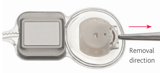
Figure 35: CI632 implant magnet cassette removal using metal tab
