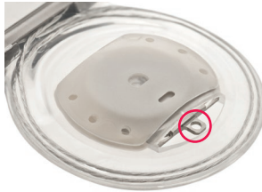
Figure 26: Metal tab on magnet cassette
