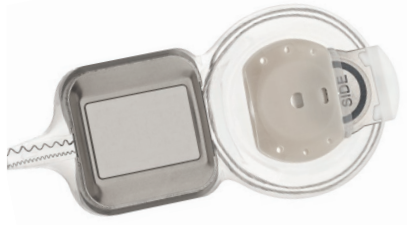
Figure 1: CI624 cochlear implant with magnet cassette partially removed from pocket
