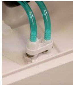
Figure 33: HPM Gas Lines Connections
