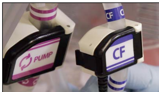
Figure 35: HPM Flow Probes
