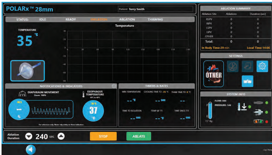
Figure 14. Therapy screen – inflation state with solid blue border when enhanced notifications are enabled
