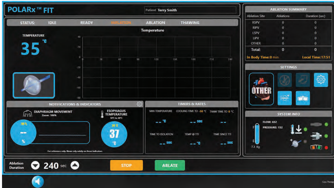
Figure 31. Therapy Screen - INFLATION state with POLARx FIT Catheter
