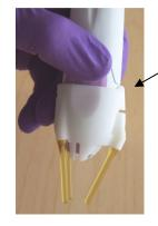
Align protrusion on the Stand-off in relation to the joint between the Handpiece and Nozzle
