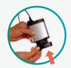
ActaStim-S will go through a self-check routine and will immediately start delivery of treatment. There is no on/off button. **Please do not insert the battery until you are ready to start treatment.**
